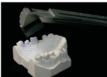
**Fig. 1** Prototype of a miniaturized single-shot intraoral 3D sensor based on the "Flying Triangulation" principle.
