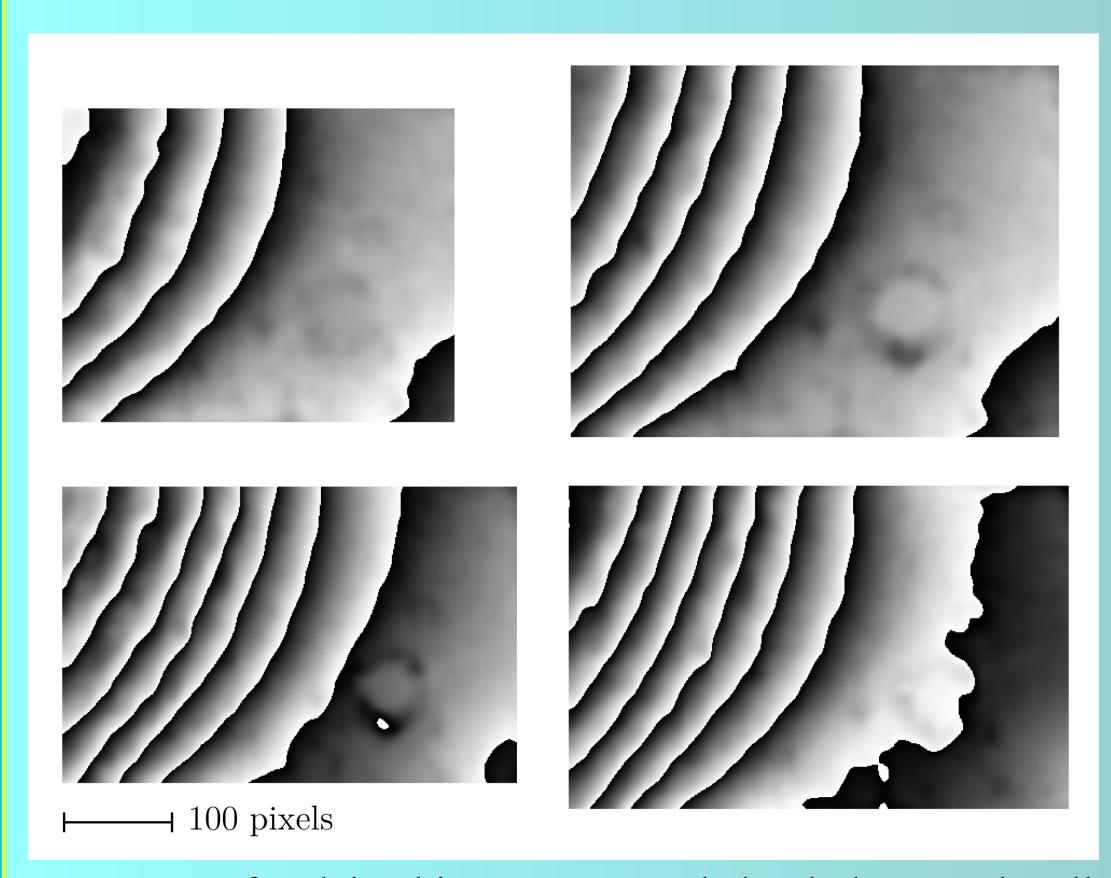
Two states of a plain object were recorded as holograms by all four cameras. After reconstructing and subtracting both states from each other, the phase-differences were calculated and unwrapped to gain values higher than  $2\pi$ . The results can be found in the figure above for each camera. The sizes of the images differ from each other due to the different positions of the CCD-chips.
