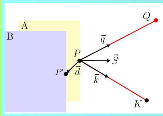
It is possible to calculate the deformation vectors  $\vec{d}$  of the deformation of an object by evaluating phase differences  $\Delta \phi$  measured, if the sensitivity vector  $\vec{S}$  is known.
