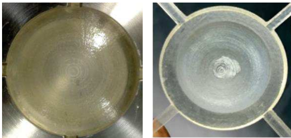
Fig. 3 Surface quality of one lens directly after the printing process.
