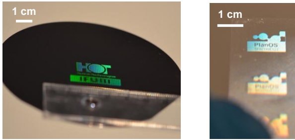
Fig. 2 Diffractive optical elements on silicon substrate (left) and PMMA foil (right).
