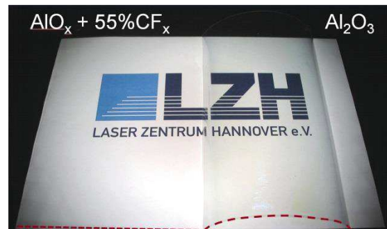
Fig. 5 : 500 nm thick AlO_xC_yF_z (left side) and Al_2O_3 coating on PMMA foil. The AlO_xC_yF_z is compatible to the foil, whereas the Al_2O_3 coating (right side) shows stress induced cracks and bends the foil.
