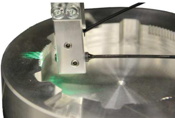
**Fig. 1** Sensor head of the fiber-optic fringe projection system next to forming tool.
