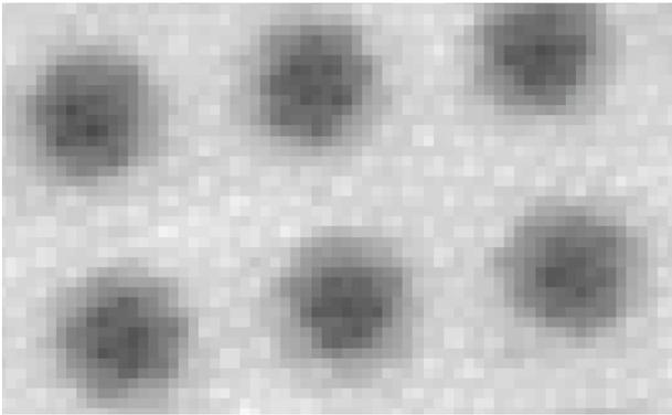
**Fig. 3** Cropped image of a point pattern (point-to-point distance:  $125\ \mu\text{m}$ ) captured through the image fiber.
