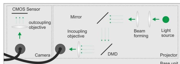
**Fig. 2** Schematic of the base unit of the fringe projection system.
