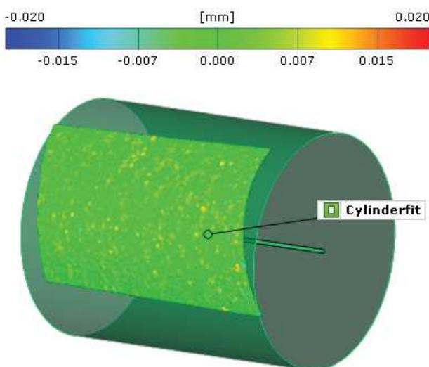
**Fig. 4** Deviation analysis (GOM Inspect) of a measurement of a cylindrical geometry.
