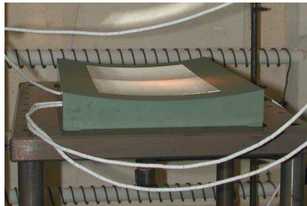
Fig. 2 Mold for Wolter-I type telescopes with a thermally formed glass mirror inside the slumping furnace
