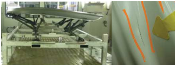
Fig. 1 Field of application: Deep-drawn parts. Left: Pre-aligned object (engine hood). Right: Constriction
