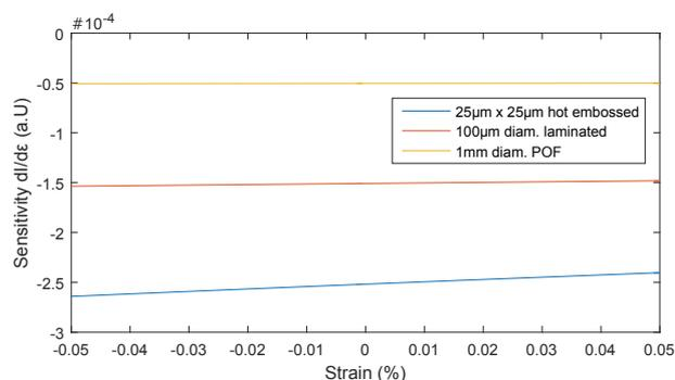
**Figure 2** Sensitivities for three different production methods of the proposed strain sensor. All sensors were calculated with a gauge length of  $l = 100\mu\text{m}$ .
