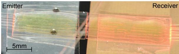
**Figure 4** Photograph of sensor prototype on the measurement setup.
