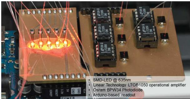
**Figure 3** Photograph of the readout electronics consisting of incoherent SMD-LEDs and a photodiode amplifier circuit.
