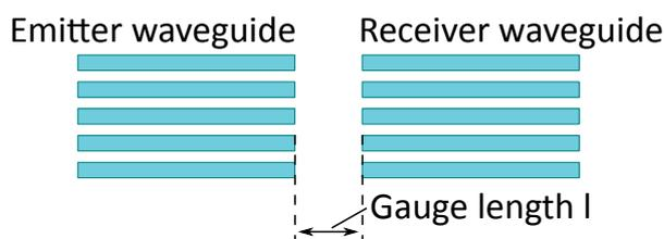
**Figure 1** Working principle of the displacement sensor.
