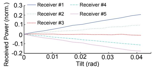
**Figure 6** Received power over tilt angle measured with the sensor system shown in Figure 3.
