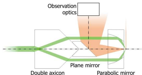
Fig. 2 Optical system for trapping (green) and observation (orange).
