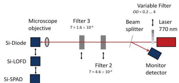
**Fig. 1** Schematic representation of the setup used for the calibration of the Si-SPAD detection efficiency.
