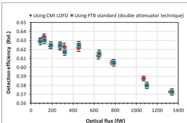
**Fig. 3** Detection efficiency of a Si-SPAD detector (PerkinElmer SPCM AQR 16) determined by using the PTB low flux measurement facility and the CMI low optical flux detector (LOFD).
