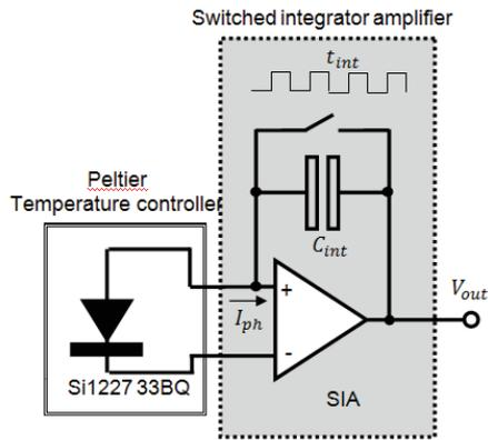
**Fig. 2** Simplified scheme of the *low optical flux detector* (LOFD).
