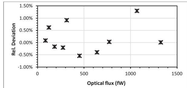
**Fig. 4** Deviation between the detection efficiency determined using the PTB's low flux facility (double attenuator technique) and the LOFD.
