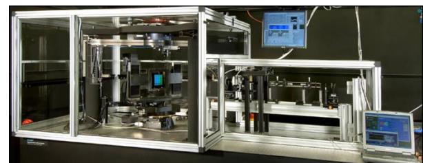
Fig. 2 Scheme of scatterometry (top) and experimental set-up (bottom) of PTB's DUV scatterometer.
