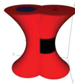
Fig. 1 CAD-Design of the SM-MM waveguide coupler with optical grating structure in the SM-waveguide (indicated by black structure).
