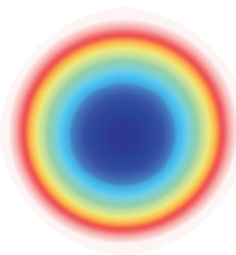
Fig. 3 diameter uncertainty due to alignment uncertainties in the measured aperture; Min(blue) = 0.09 nm / Max(white) = 0.23 nm
