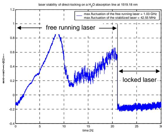
**Figure 4** Stability of the WMS-technique on the 1519.18nm-H<sub>2</sub>O absorption line.
