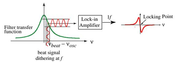
**Figure 5** Evaluation of the first harmonic on an electrical low-pass filter with Lock-In detection.
