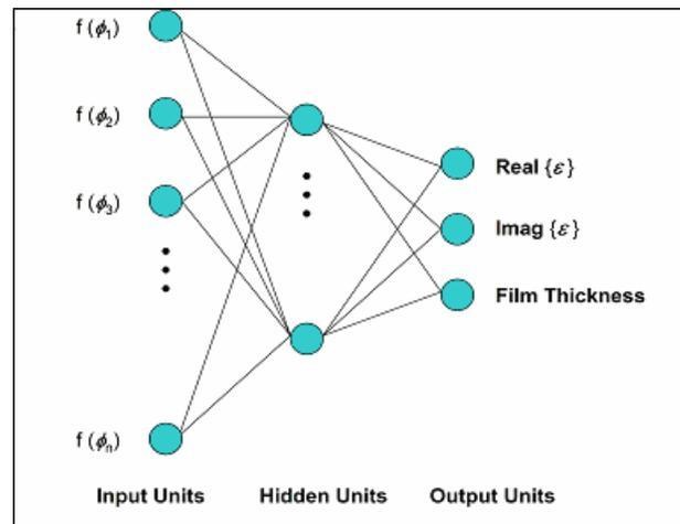
**Fig. 1** EBPN structure with '40' input units and '3' output units,  $f(\phi_i)$  is the value the reflection data for the incidence angle  $\phi_i$  at a fixed wavelength.
