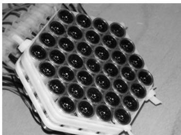
**Fig. 2** Sound source consisting of 37 piezoelectric transducers of 16 mm diameter each
