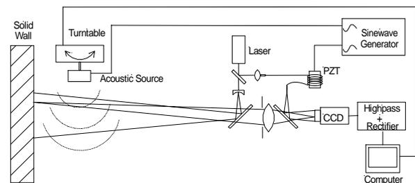
**Fig. 1** Schematic of ESPI set-up for the measurement of sound fields
