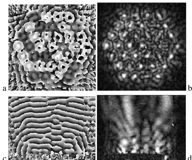
**Fig. 3** Tomographic analysis of 38.5-kHz ultrasound field above an array of 37 piezoelectric transducers, assembled without correction of their phases. a and b: phase and amplitude in a plane parallel to the array and directly above it. c and d: in a plane perpendicular to the array and through the centers of the lower row of transducers
