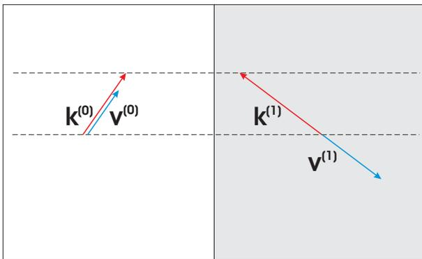
**Fig. 1** Negative refraction at an interface. Incident (refracted) wave with wave vector  $\vec{k}^{(0)}$  ( $\vec{k}^{(1)}$ ) and group velocity  $\vec{v}^{(0)}$  ( $\vec{v}^{(1)}$ ). The direction of a light ray is given by the group velocity vector.
