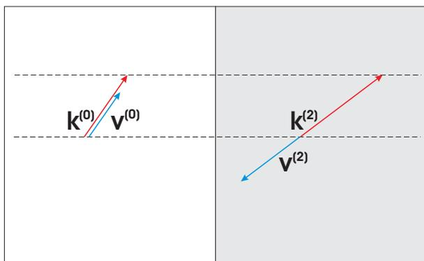
**Fig. 2** Positive refraction at an interface. Incident (refracted) wave with wave vector  $\vec{k}^{(0)}$  ( $\vec{k}^{(2)}$ ) and group velocity  $\vec{v}^{(0)}$  ( $\vec{v}^{(2)}$ ).
