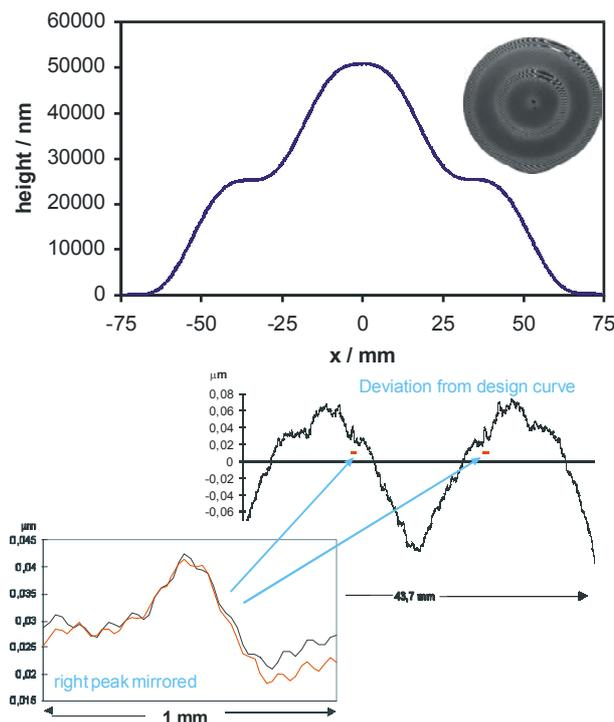
Fig. 6 TMS measurement of a diamond-lathed surface, manufactured by PTB's Working Group 5.53 "Advanced Fabrication Technology."
