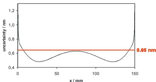
Fig. 5 Uncertainty of a single measurement corresponding to the model. 16 sensors, 750 scan steps, sensor distance 0.2 mm (= lateral resolution). Assumed noise: distance sensors 1nm, autocollimator 0.25 nm/mm (0.05 arcsec).
