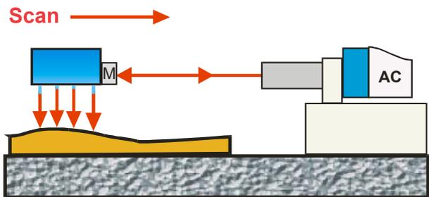
Fig. 2 TMS system with multiple distance sensor and autocollimator as tilt sensor.
