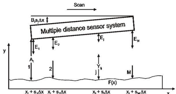
Fig. 3 Some properties of the mathematical model. A, B: height and tilt offset at the sensor system position, E: offset error of single distance sensor, F: topography of specimen.
