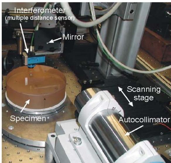
Fig. 4 Test set-up for TMS measurements.
