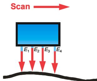
Fig. 1 Four-sensor system with systematic sensor offset errors  $E_1 \dots E_4$ .
