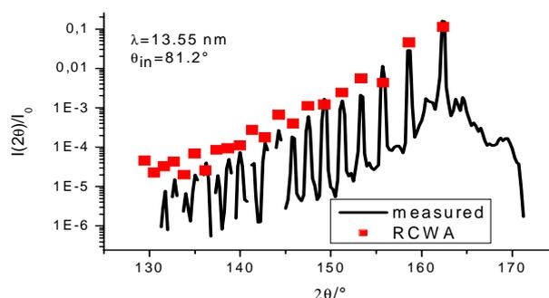
**Fig. 5** Measurements on the CoG1 mask @  $\lambda=13.55$  nm. The simulated data has been scaled by a factor of 0.6.
