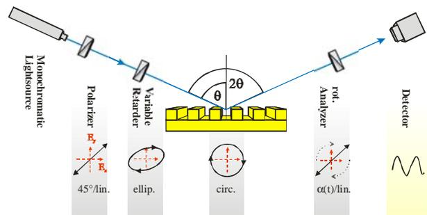
**Fig. 1** Ellipsometric Scatterometer for measuring  $\Psi$  and  $\Delta$  of the 0<sup>th</sup> diffraction order. Here the PSCA configuration (Polariser, Compensator, Sample, and Analyser) with rotating analyser is sketched. At a standard scatterometer the polarising elements are lacking and the detector scans the diffraction pattern.
