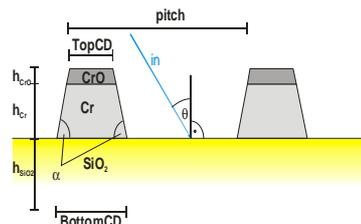
**Fig. 2** Scheme of the periodically structured CoG masks as they are used here for simulations and measurements, respectively.
