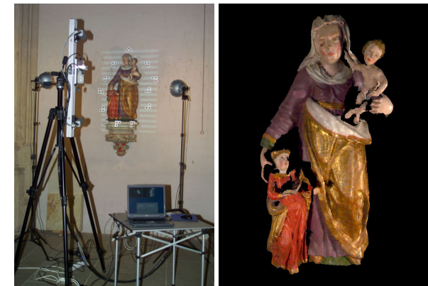
Fig. 4 3-D measurement of a Madonna statue in the Lamberti Church in Münster with a mobile true color topometric sensor and the 3-D data with calibrated color information of the measurement (approx. 200.000 triangles with textures).
