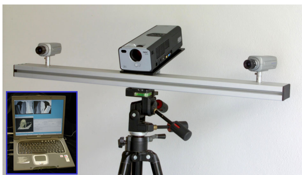
Fig. 1 Setup of the topometric sensor: the 3-D coordinate measuring system uses a DLP video projector for fringe projection and high-resolution color CCD cameras for image capturing; the mobile system is controlled by a notebook.
