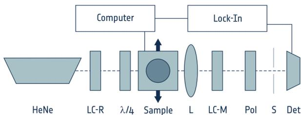
Fig. 1 Illustration of the optical arrangement for the measurement of the stress induced phase shift.
