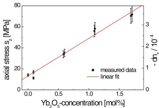
**Fig. 4** Maximum mechanical stress in the core for different  $\text{Yb}_2\text{O}_3$ -concentrations.
