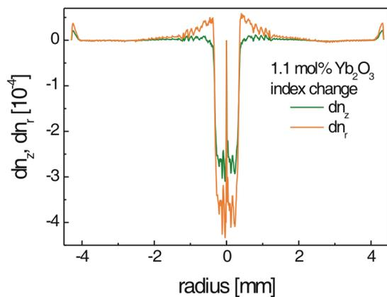
**Fig. 5** Calculated radial index shift  $dn_r$  in comparison to the axial  $dn_z$ .
