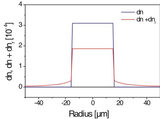
**Fig. 6** Step index profile with an NA of 0.03 (blue line) and the calculated stress changed index profile (red line)
