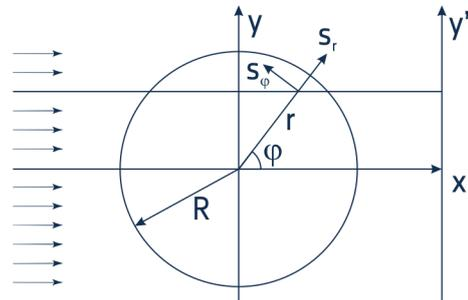
Fig. 2 Definition of the used coordinate system;  $s_r, s_\varphi$  - stress components.
