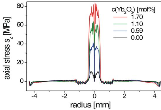
**Fig. 3** Axial stress component  $s_z$  of four samples with different  $\text{Yb}_2\text{O}_3$ -doping.
