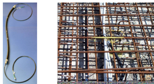
Fig. 1 Fiber Bragg-sensor designed for civil structure monitoring (AOS GmbH, Dresden and CORRSYS 3D Sensors AG, Wetzlar: Hausertorbrücke, Wetzlar).
