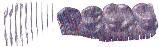
Fig. 5 Left: Several unregistered 3D views in the sensor coordinate system. Right: Complete and dense 3D model after automatic registration.
