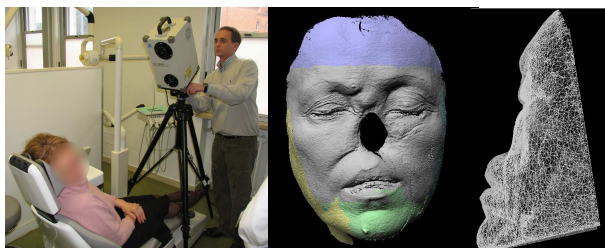
Fig. 3 Fabrication of the nose prosthetic replica. Left: acquisition of the patient's face; Center: aligned point clouds of the whole face; Right: triangle mesh.
