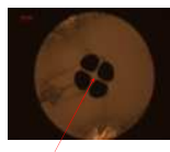
The central hole selectively filled with Epoxy-DR1
