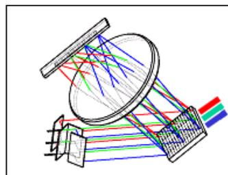
**Fig. 3** Spectral pre-selection by dichroic filters and structure-modulated diffraction grating.
