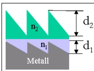
**Fig. 2** Material-dispersion tuning achieved by a reflective double-grating.
