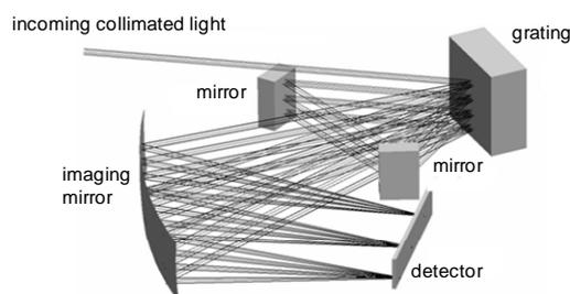
**Fig. 1** Recycling loop of the zeroth-order specular false light of a blazed grating.
