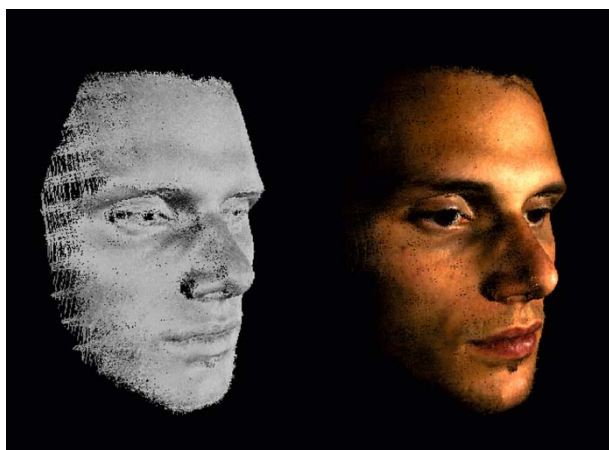
Fig. 4 Acquired 3D model before and after the texture mapping sequence.
