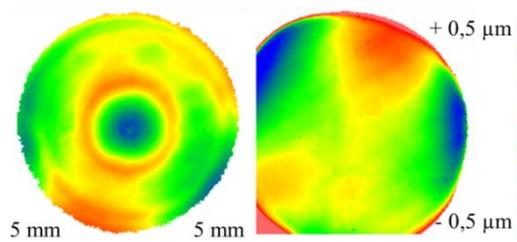
**Figure 3:** Measurement of the curved and the planar side of the laser polished lens of fused silica.
