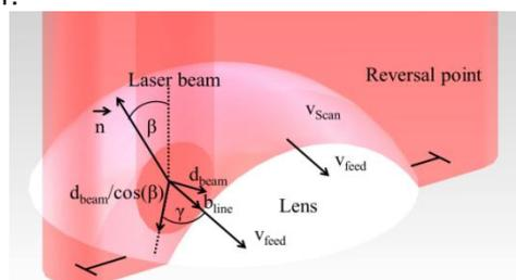
Figure 2: Sketch of the non-perpendicular incidence of the laser beam on a lens
