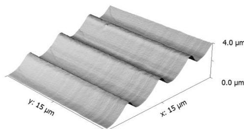
**Fig. 4** AFM-Scan of a grey scale structure at a surface angle of 15°.
