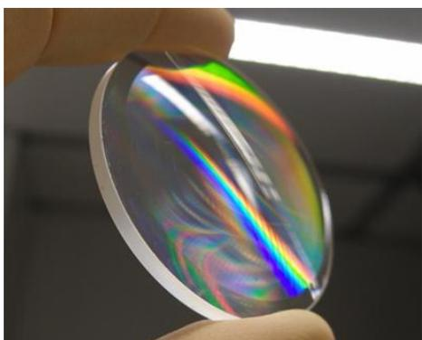
**Fig. 3** Photograph of a spherical lens with binary Fresnel zone plate structure: max. slope angle: 15°, min. structure period: 2.4µm
