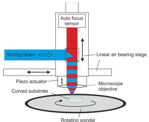
Fig. 1 Schematic of the writing head
