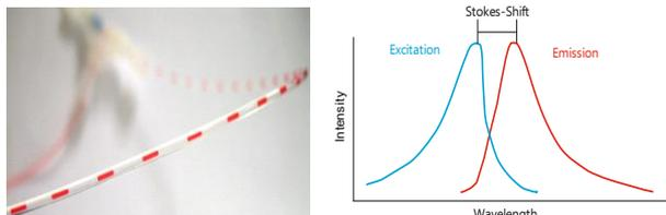
**Fig. 1** Left: Dye solution with carrier media Tetradecane as compartments in a tube. Right: Functional principle of fluorescence detection [1].
