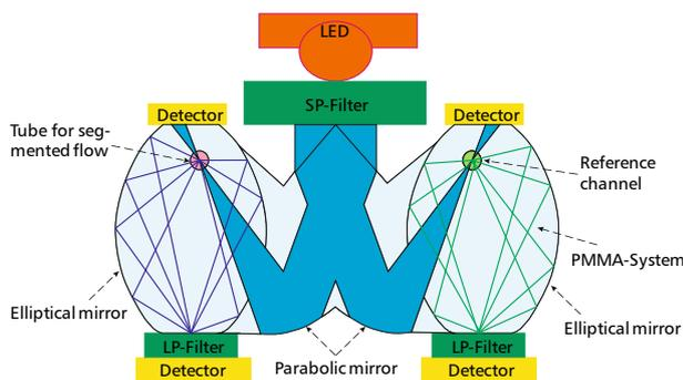
**Fig. 3** Schematic setup of the fluorescence detector.
