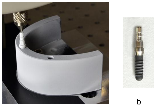
Fig. 4 (a) Model of a jaw (with inserted dental implant). (b) Dental implant
