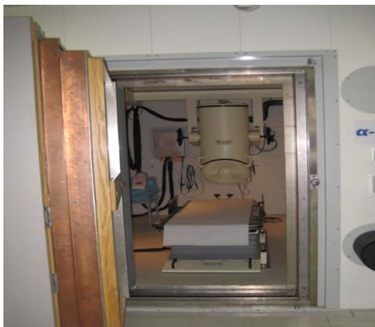
Fig. 3 MEG inside its magnetically shielded room (MSR).
