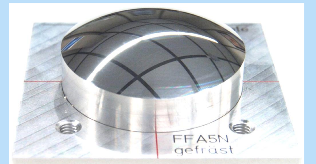
Free-form surface with diamond turning grooves
