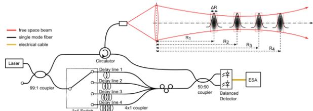
Fig. 3. Illustration of CW Lidar concept with range independent probe length
