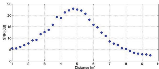
Fig. 6. Experiments result of the SNR for different target distance with a 7m fiber delayline
