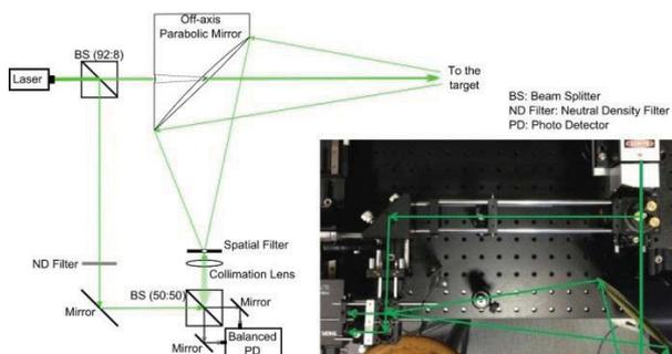
Fig. 4. A free space monostatic un-confocal Doppler wind Lidar system design for experimental testing
