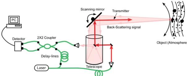
Fig. 1. Concept of a Doppler wind Lidar system
