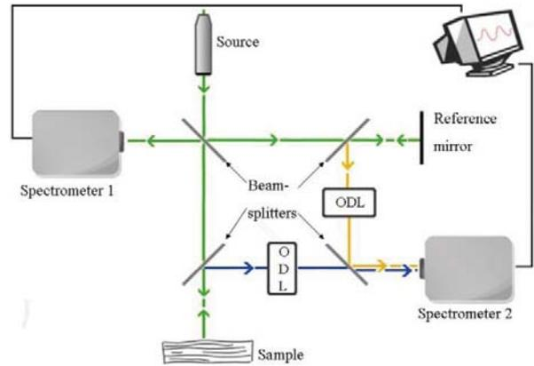
Fig. 2. OCT system for paper quality measurement [4]
