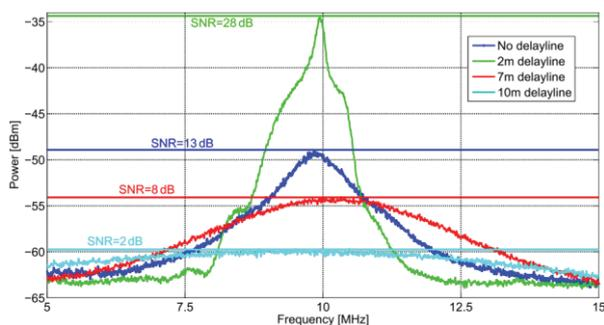
Fig. 5. Doppler spectrum with different delayline lengths for measuring at a target distance of 2m
