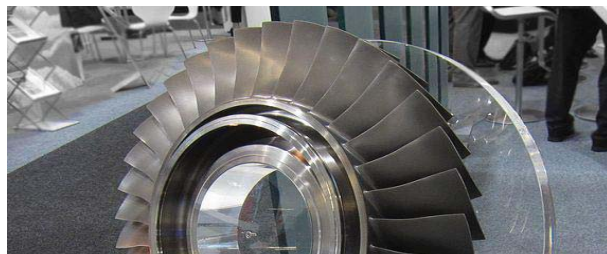
Abb. 2 Blade Integrated Disc (Blink) (by Olivier Cleynen - CC BY-SA 3.0)
