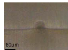
Fig. 2 Cross-section of an embedded multimode waveguide integrated in a PMMA cladding
