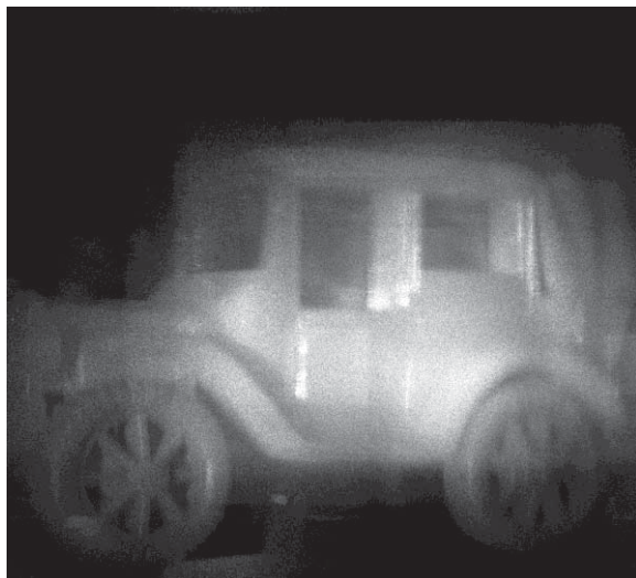
Fig. 4 Reconstruction of a digital hologram of an object taken under doubled resolvable angle in vertical as well as in horizontal direction
