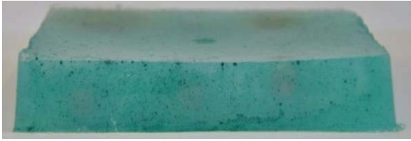
Fig. 2: Silicon phantom made out of soft silicon ZA00 and Phthalogreen particles for better detection of the displacement.
