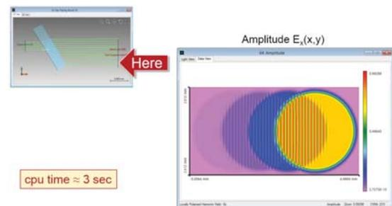
**Fig. 4** Non-sequential zigzag waveguide modeling with geometric field tracing including interference of decoupled light.
