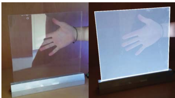
Fig. 1 The EVONIK PLEXIGLAS LED left: without illumination highly transparent, right: illuminated as homogeneously diffused luminaire, caused by integrated scattering nano-particles
