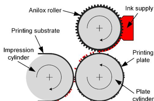
**Fig. 2** Flexographic printing unit.
