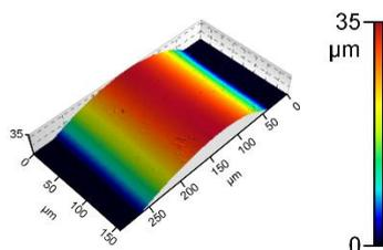
**Fig. 3** Confocal microscopy of printed waveguide; 10 layers of acrylate.
