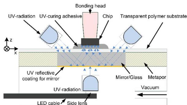
**Fig. 4** Schematic of optodic bonding.
