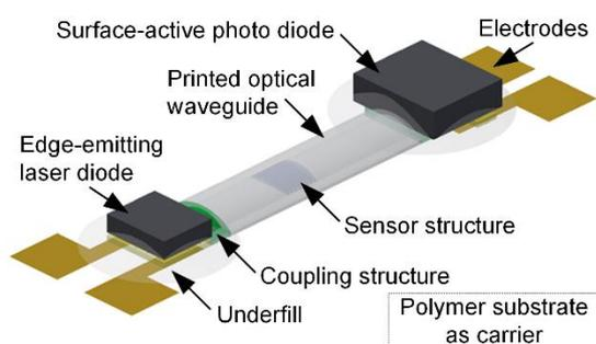
**Fig. 1** Planar optronic sensor system consisting of printed waveguide with integrated sensor structure, laser diode and photo diode.
