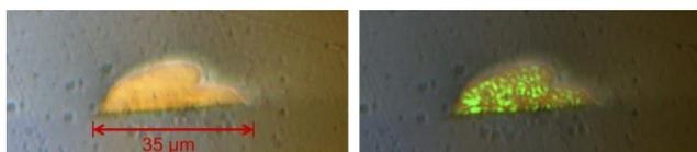
**Fig. 3:** Light guiding test, not illuminated end facet (left), intensity pattern with encoupled light beam (right)
