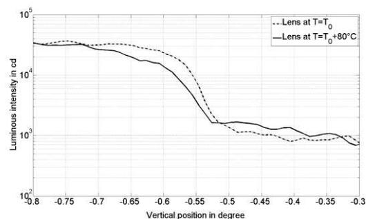
**Fig. 9** Section through the cut off line at  $x=-0,5^\circ$  of the light distribution based on the kitted lens doublet at two different temperatures
