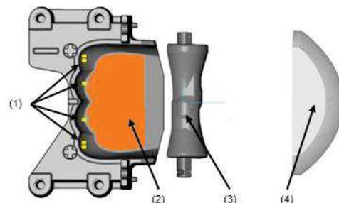
**Fig 1** Top view of a projection headlamp system containing light sources (1), a free-form reflector (2), a cut-off aperture (3) and an aspheric lens (4)
