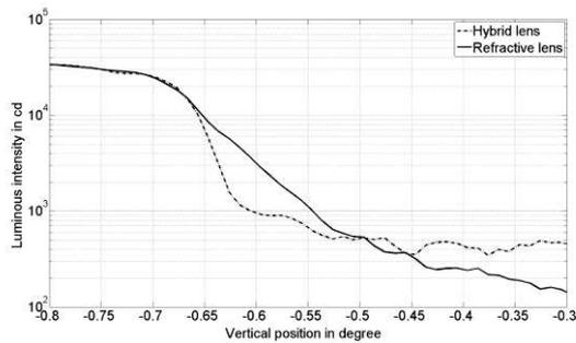
**Fig. 4** Section through the cut off line at  $x=-0,5^\circ$  of the light distribution based on a hybrid lens and on a refractive lens
