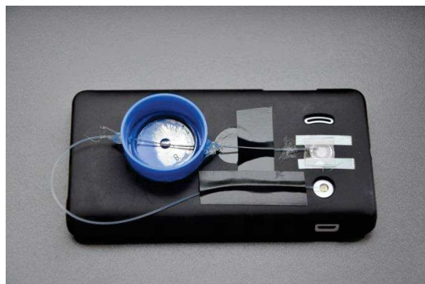
Fig. 7 SPR sensor system developed for the high sensitive refractive index sensing using a smartphone.
