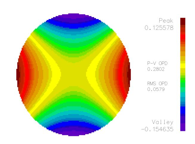
This astigmatism splits the axial horizontal and vertical waist positions and generates an elliptical beam profile. Very close to the best focus position the orientation of the ellipse changes from horizontal to vertical, and the beam profile becomes circular:
