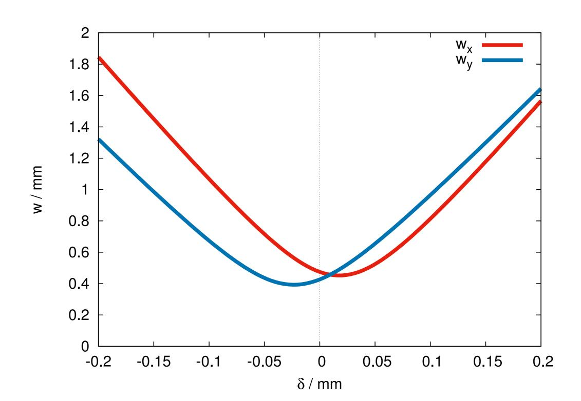
The small deviation of the position with the most circular beam profile from the best focus position can be corrected subsequently. The visual detection of this circular beam profile is even more sensitive than the search of the minimum waist radius.
