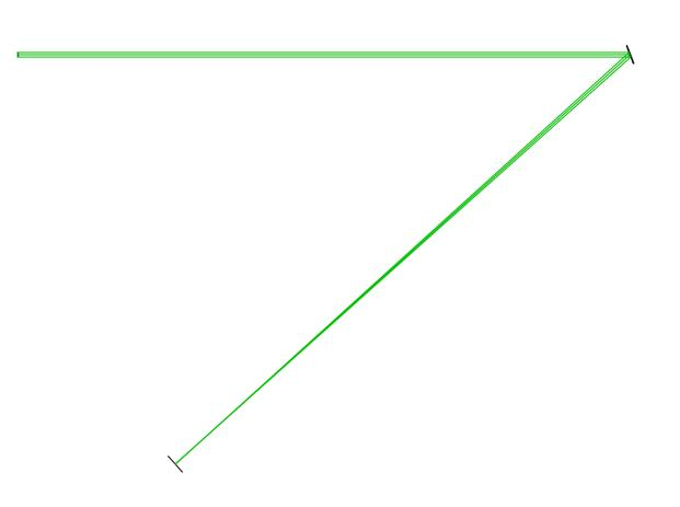
Due to the off-axis use the mirror introduces significant astigmatism:
