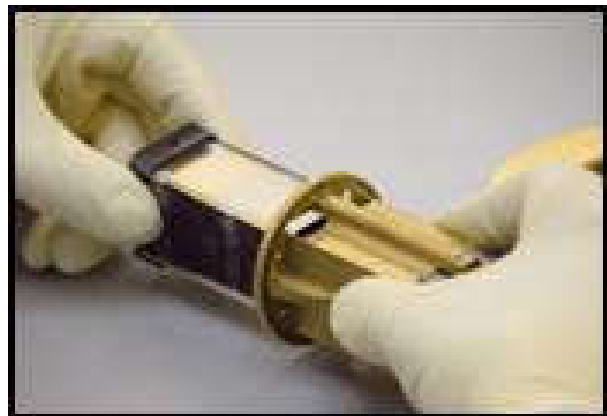
Fig. 1: The lobster eye optical module for the VZLUSAT1 Cubesat satellite [1].
