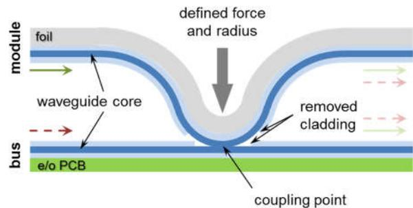
Fig. 1 Principle for an asymmetric optical bus coupler
