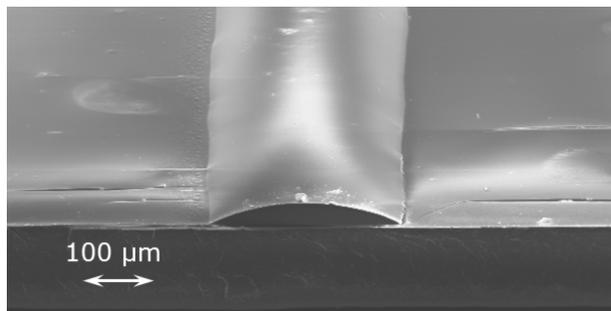
Fig. 3 REM image of an aerosol jet printed waveguide core
