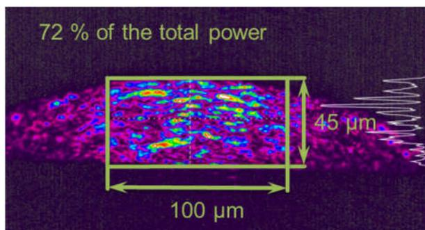
Fig. 4 Near field image of the end face of an aerosol jet printed waveguide with the area including 72% of the total input power
