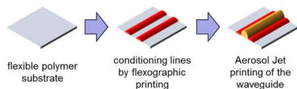
Fig. 2 Process steps for the waveguide manufacturing
