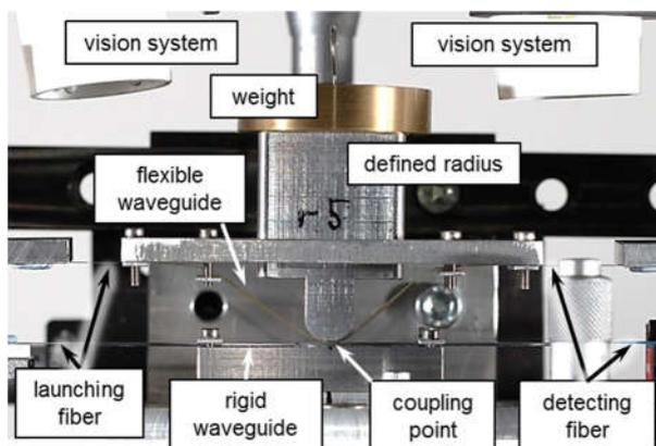
Fig. 5 Measurement setup for the coupling experiments
