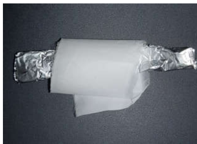
Fig. 2 Sample of an electro spun fiber mat. The sample consists of polymer fibers with diameters of 2-5 \mu\text{m} . Due to the fabrication process the fibers are oriented predominantly in one direction, not visible to the eye.
