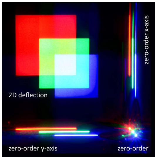
Fig. 2 The wavelengths 450 nm, 320 nm and 638 nm are deflected onto a screen by two AODs in their full deflection range. As a result a 2D deflection regime can be observed with a wavelength-dependent angle separation. There are zero-order beams that pass the AODs without deflection.
